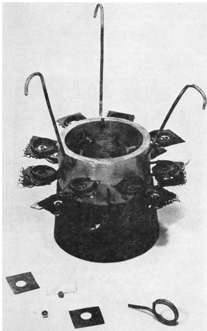
Fig. 2. Assembly for supporting layers during melting point determination.
